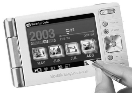
The top of Kodak's digital camera line, the EasyShare One, makes a wireless connection to the Internet to email photos without a computer — but it includes a throwback to the company's Auto-graphic folding cameras of a century ago: a stylus to write captions on the camera's back.
