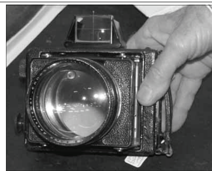
A lovely pigskin covered Frena, designed by Joseph Clarke and made by Beck in 1892. This was the first "automatic" camera to use packs of celluloid cut film ("like a pack of cards") for up to 40 exposures.
