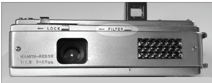
pop-out viewfinder had parallax correction, and the shutter speed range was B 1/2 - to 1/200<sup>th</sup> second. A built-in slide-in filter holder was activated by a small lever on the front of the camera.
