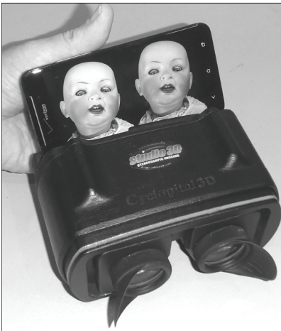
Digital phone slides into the back of the HD3D View-Vaster
