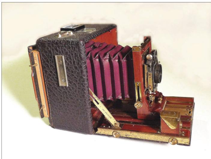
The newly repaired model camera shown above has a brass Century label but no model markings. The 4 x 5 field camera is most likely from the 40 series, probably 40—43. It has a leather covered wood body and red leather covered bellows. The interior is red mahogany with nearly all the metal parts
