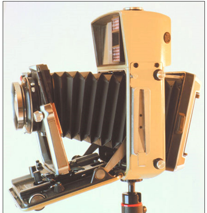
Technika 70 with dropped bed, maximum front rise, lens and rear standards tilted back to maximum. Camera back can be adjusted for four-way swing, https://www.shutterbug.com/content/classic-camerasbrthe-linhof-technika-70
