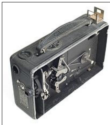
Open view of the earliest version of the Ciné-Kodak Model B https://tinyurl.com/3hbkvk8t
